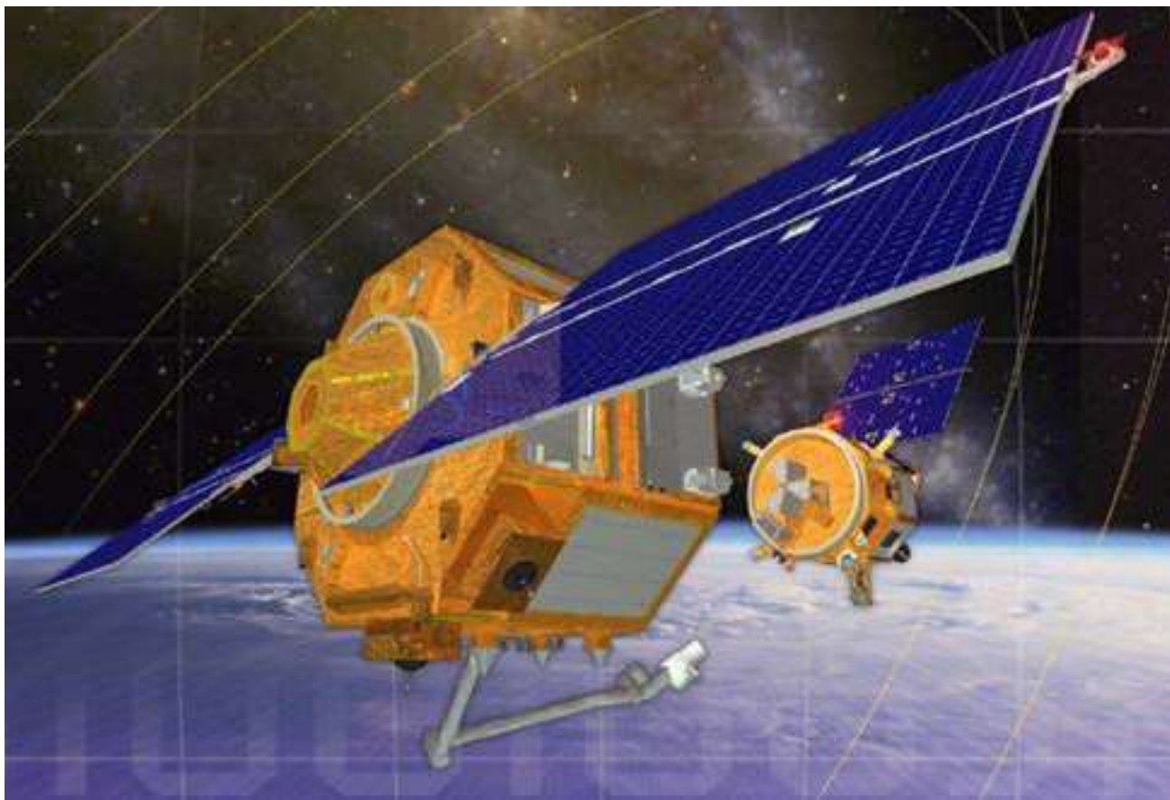
The Orbital Express program proved the concept of robotic satellite repair, refueling, and maintenance on orbit.
